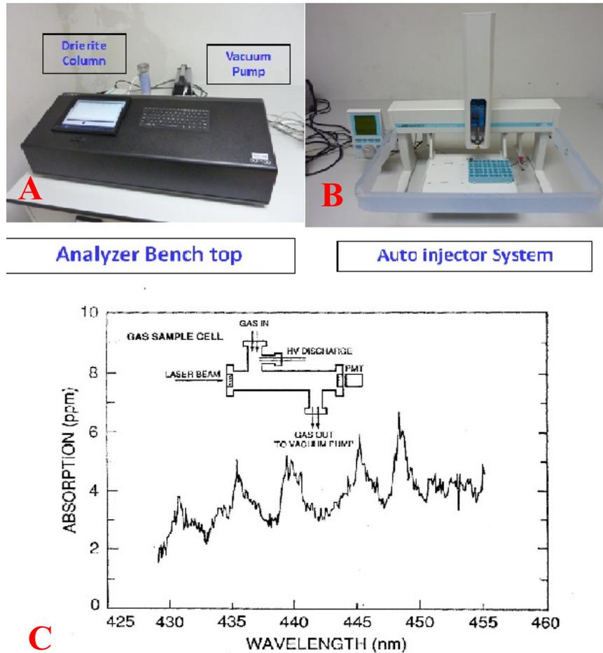
Fig. 3 Liquid Water Isotope Analyzer details showing the analyzer bench top compartment (A), the auto ejector compartment (B) and the analyze concept diagram with laser absorption characteristic from O'Keefe and Lee, 1989 (C).
